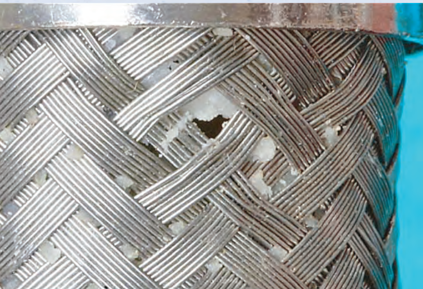
FIGURE 3: Eventually and inevitably environmental conditions cause the inner tubing to degrade from the inside out and fail.
